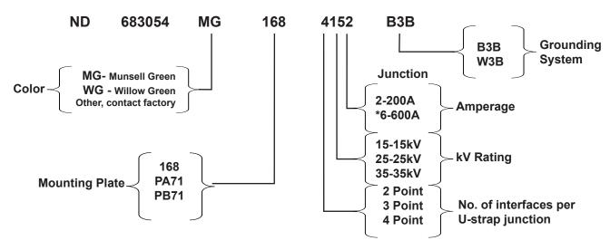
\*This cabinet will accommodate 15-35kV, 200 & 600Amp junctions with U-straps. It will accommodate 200Amp taps off the 600Amp deadbreak junction. It wil also accommodate Cooper 35kV 200/600Amp loadbreak junctions.
