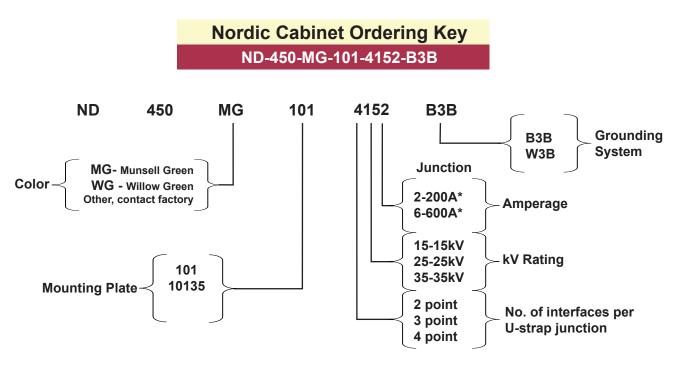
\*This cabinet will accommodate 15-35kV, 200 & 600Amp junctions with U-straps. It will accommodate 200Amp taps off the 600Amp deadbreak junction. It will also accommodate Cooper 35kV 200/600Amp loadbreak junctions with the 10135 mounting plate only.
