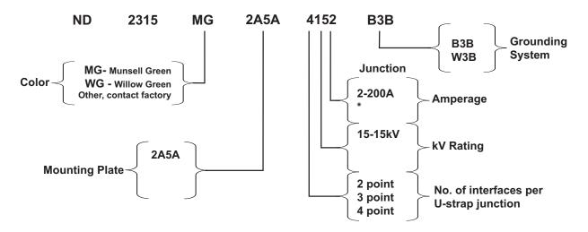
\*This cabinet will only accommodate 15kV 200Amp loadbreak junctions with U-straps.
